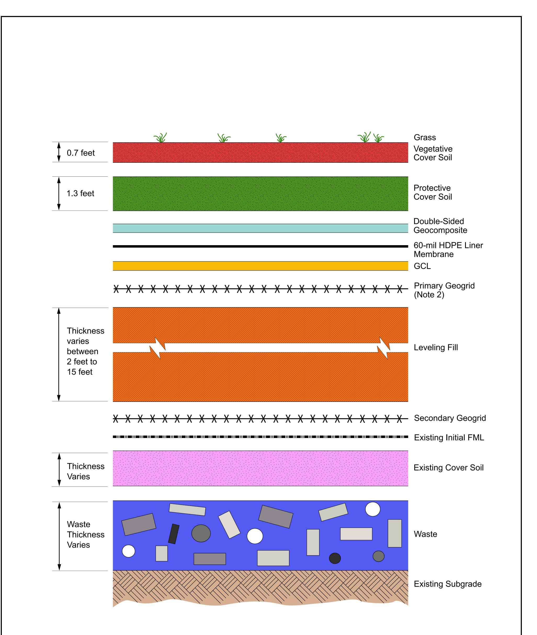
Note 1: Spacing between geosynthetic layers and other layers is exaggerated in order to fully visualize the layers.
